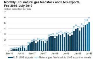
feedstock deliveries to LNG export terminals averaged 5.5 Bcf/d in June and 6.0 Bcf/d in July, implying a 14% and a 15%, respectively, loss on conversion of gaseous natural gas into liquefied natural gas (i.e., 14% and 15% of natural gas feedstock was used as fuel in the liquefaction process).
